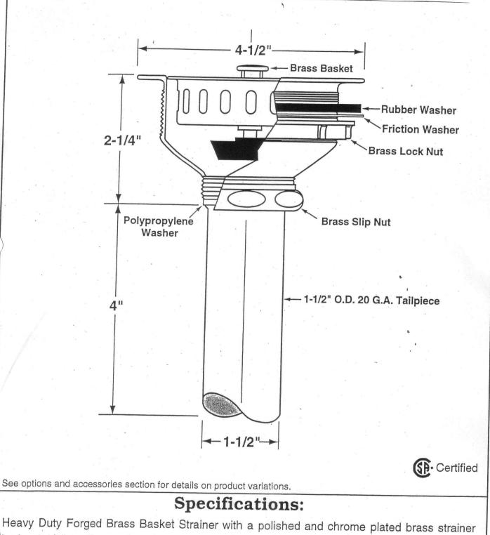
body, 1-1/2" x 4" seamless brass tailpiece, cast brass lock and coupling nuts. Fits sink thickness up to 3/4 inch. Basket Strainer shall be in compliance with CSA or other recognized testing authority and bear both manufacturer and testing mark.
