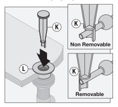
**Note:** Stopper can be installed removable or non-removable determined by eye hole position.
