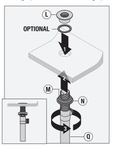
**Note:** Make sure drain cavity (on drain body) faces rear of sink.
