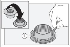
Insert flange (L) into drain opening.
