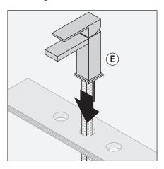
1b) **SLS-3622:** Insert faucet body (E) through deck plate (Z) and deck surface.
