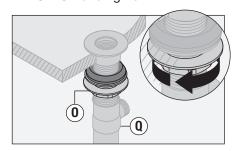
**Note:** Make sure flange is centered in drain opening.
