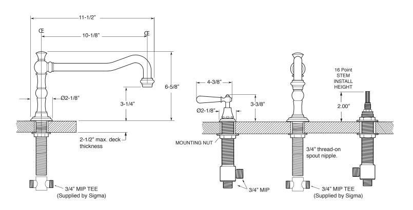
NOTE: Spout and valves install through 1-1/4" diameter holes.
