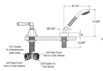
Spout and valves install through 1-1/4" diameter holes.
