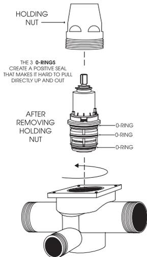
To remove cartridge from body: Rotate cartridge counter clockwise only.
