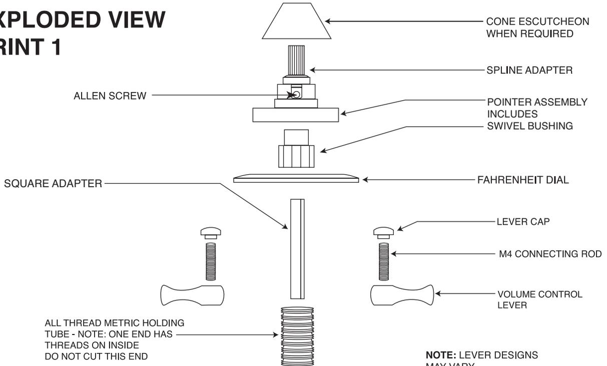
ALL THREAD METRIC HOLDING TUBE - NOTE: ONE END HAS THREADS ON INSIDE DO NOT CUT THIS END
