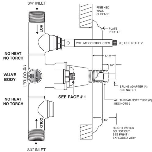
**INSTALLER NOTES:** THIS VALVE MUST BE INSTALLED AS SHOWN ABOVE
