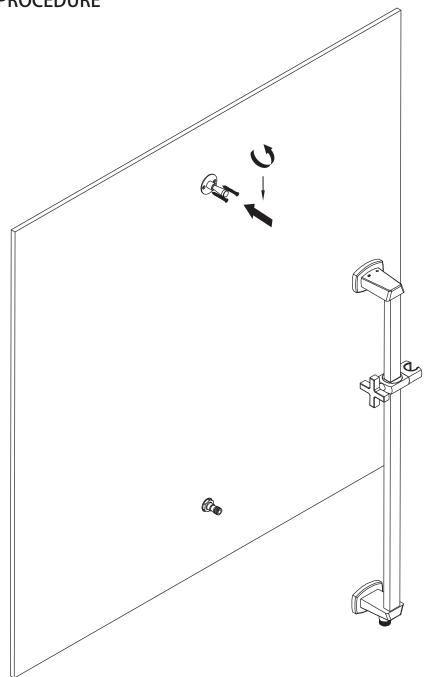
Bring out supplied 1/2" connection and install top slide on connector with supplied screws
