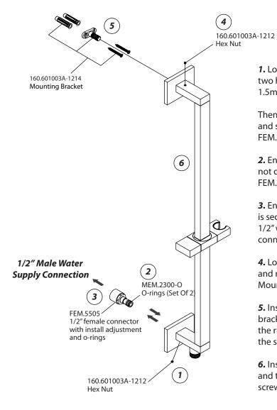
1. Loosen & remove two hex screws using 1.5mm Allen key.
