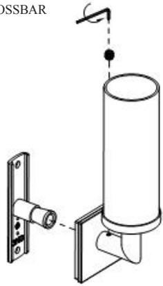
② MOUNT CROSSBAR TO ELECTRICAL BOX (NOT INCLUDED) USING #8 SCREWS.
