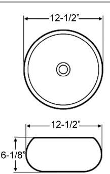
Dimensions of fixture are nominal and may vary within the range of tolerances established by AMSE Standard A112.19.2.2013 Dimensions and specifications subject to change without notice.
