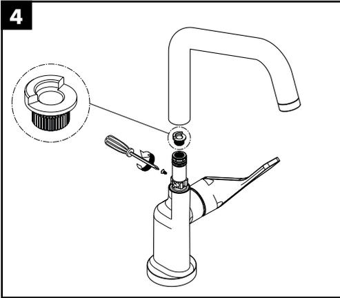
With the spout cam in place, the spout will rotate  $75^\circ$  to the right, and  $75^\circ$  to the left of center.
